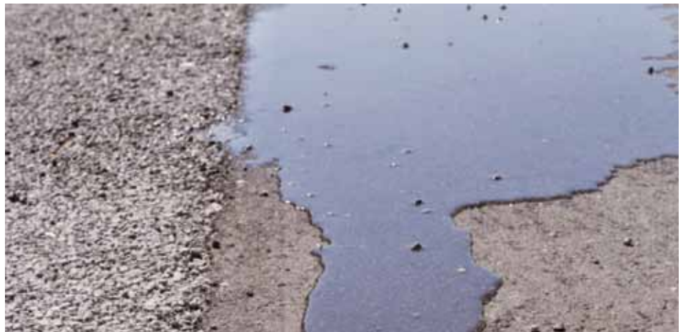
(above) By changing the size ratio of the gravel used, permeable concrete sets with large empty spaces between the aggregate, allowing rainwater to pass through the pavement.
