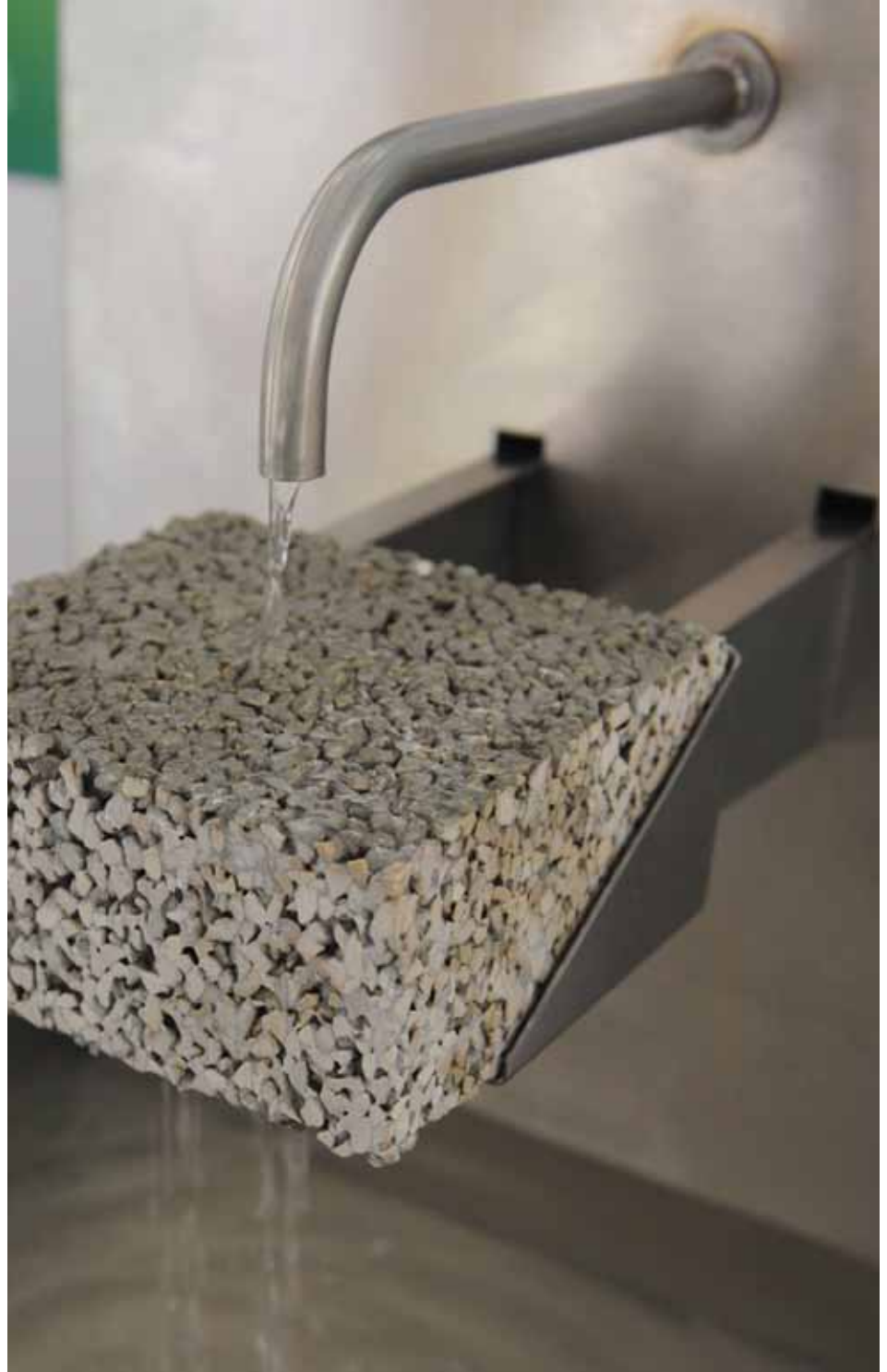
(above) Permeable concrete is an innovation in paving technology that allows rain water to flow through paved surfaces.
